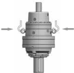
Levage et manutention corrects
